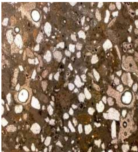
Fig.(26 ) Oolitic grainstone Quartz , grain Calcite ,spary calcite structure peloids , structure less peloids, Superficial Ooides Composite Ooides ,and shell fragments.
