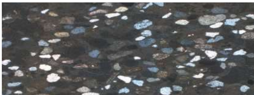
Fig.(25 ) P.m. view of limestone Spherical Quartz grains , Calcite , microcline, shell fragment and high porosity before compaction X40
